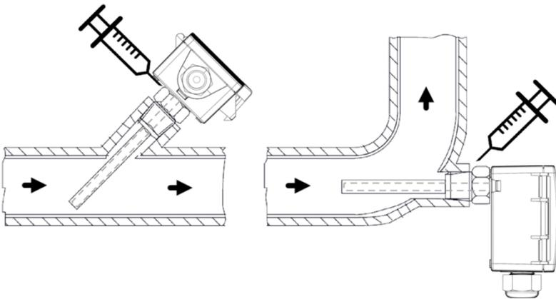
Mounting with immersion pocket or compression fitting for usage in liquid media. Use contact fluid for better heat transfer between sensor and measuring medium.
