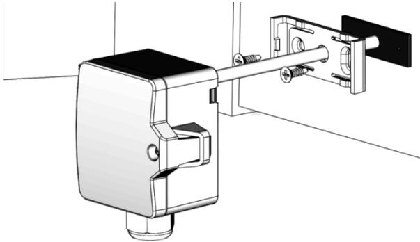
The sensor can be mounted on the ventilation duct by means of the mounting clip. For risk of condensate permeation in the sensor tube respectively in the immersion pocket the bushing must be installed in a position that occurred condensate can run off.
