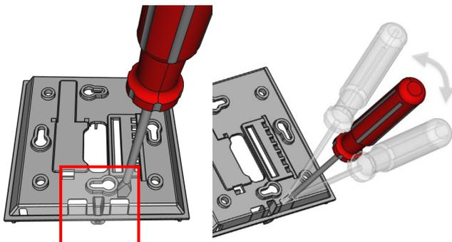
On the upper side of the base plate there are 2 grits as position for a drill hole max. Ø 6 mm
