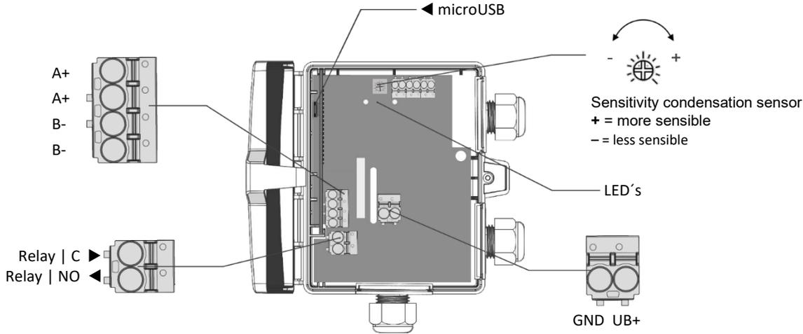
The relay is energized in the operating state (relays NO and C connected). Upon dew permeation or when the operating voltage is switched-off, the relay falls off.
